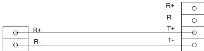
Figure 2: (Left) PTZ Connections. (Right) Encoder Serial Connector
